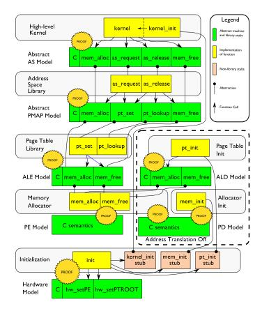
Fig. 3. Complete Plan for VMM Certification
