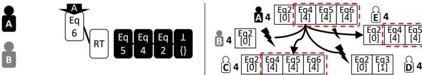
(f) ADO push and multi-Paxos phase 2 partial success due to a network failure (Eq4 and Eq5 are successfully committed to a quorum consisting of A, C and E, but Eq6 is not fully committed).
