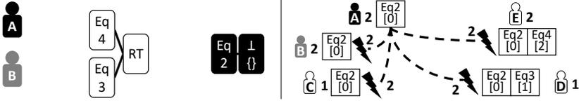
(a) ADO pull and multi-Paxos phase 1 failure due to a network disconnection.
