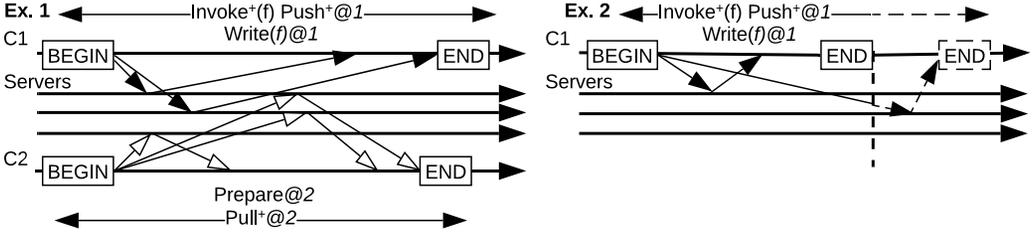
**Fig. 14.** Asynchronous networks complicate ordering and determining event completion. Examples show Paxos-like systems where successful operations require support from a majority of servers (2 out of 3). Diagonal arrows represent communication in physical time. Dotted arrows represent future events.
